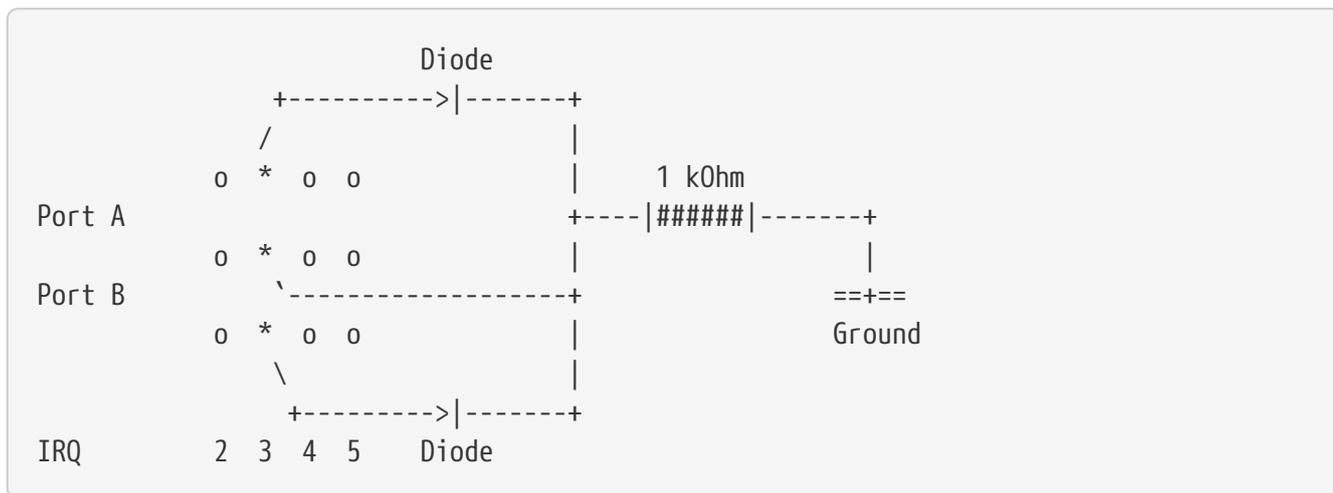
The cathodes of the diodes are connected to a common point, together with a 1 kOhm pull-down resistor. It is essential to connect the resistor to ground to avoid floating of the IRQ line on the bus.
